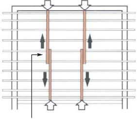
Brace lapped over 2 trusses
